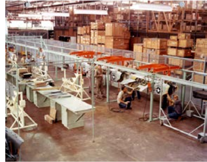
The ADM-20 Quail missile, here undergoing repair at Oklahoma City, 1962, was to serve as a decoy to confuse enemy radar tracking US bombers.
